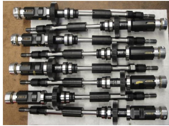
Cartridge Spindle Units, supplied for a 16-spindle installation.
