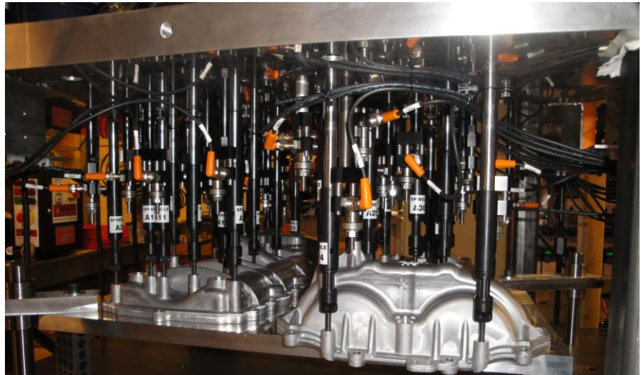
This Multi-spindle Head verifies thirty-nine M6 blind holes simultaneously. Compliant toolholders accommodate X-Y and angular positioning errors. Thread depths are individually set with fingerwheels, and a set of thread depth masters were supplied for this job. The parts here are automotive Cam Covers.
