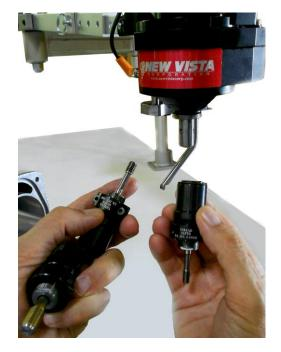
New Vista's new **Type FP Toolholding System** will accommodate any size or depth of thread.
