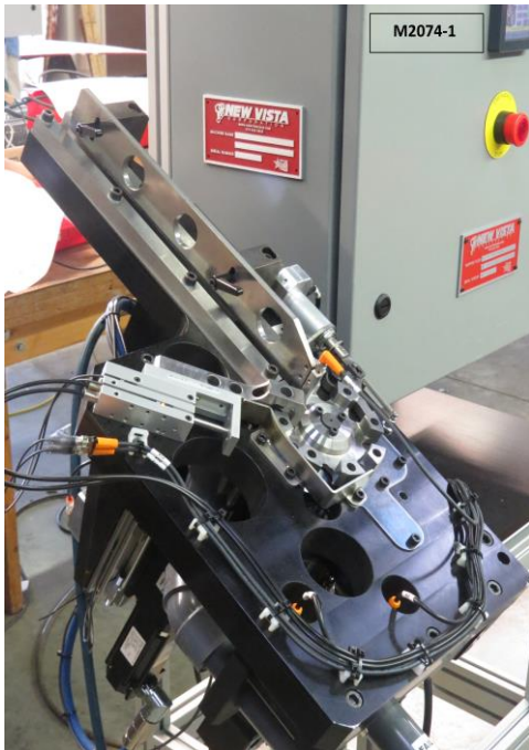
IND-STH verifying M14 internal threads in automotive sensor bosses.
