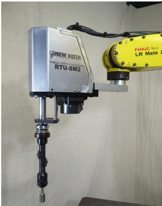
An RTU-SM2 with mounted Supercompliant Toolholder. This arrangement will pick up holes that are \pm 1 mm out of position and angularly mispositioned as well — and gage them as if they were positioned perfectly.
