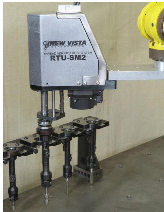
An RTU-SM2 approaching a New Vista Type J Tool Dock. The two tools at the left are for thread gaging. The two at the right are for thread remediation — chasing out existing threads.
