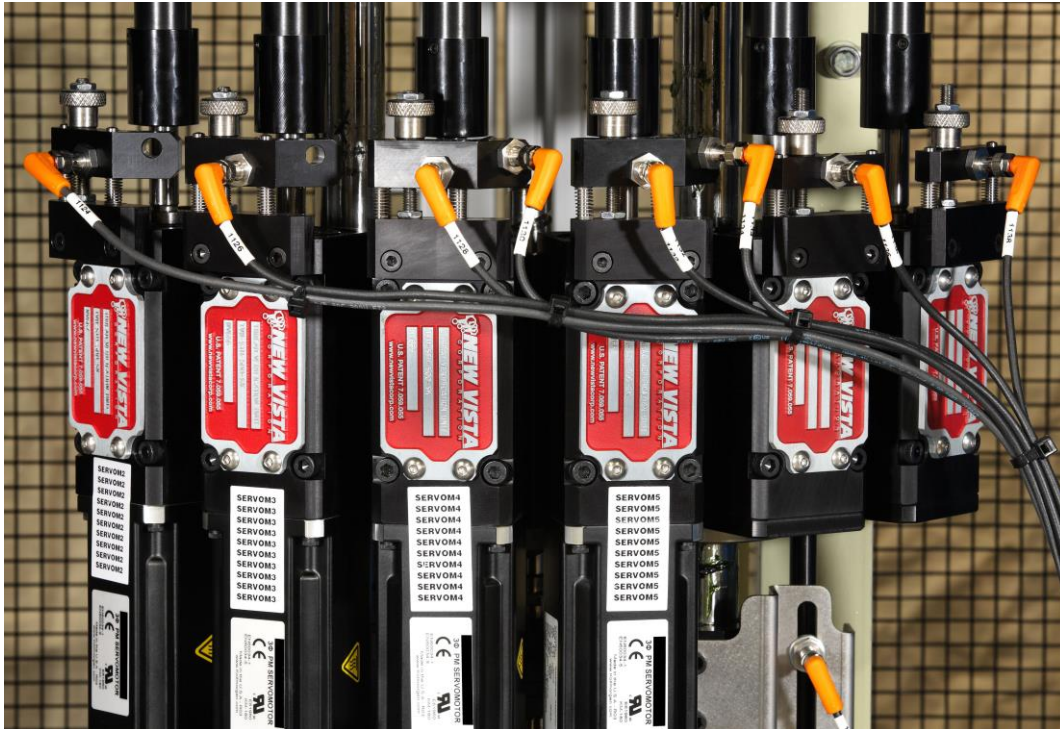
SHOWN: Bank of servo-driven STHs for oil filter application.
