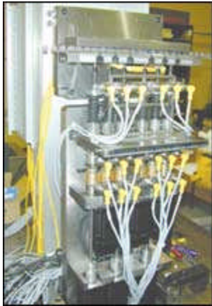
Parts are delivered to the inspections machine across the top. The six servo-driven gages inspect six parts at a time.
