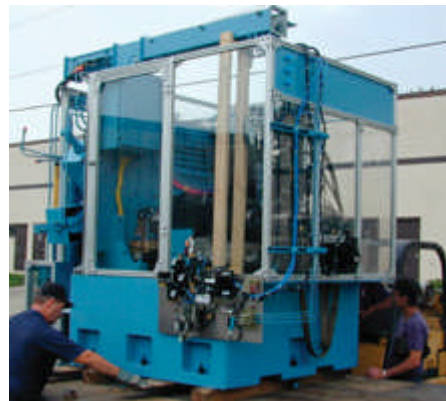
As-cast polymer composite base for high-production automated groove and trim machine (left), and finished machine being rigged for shipping.
