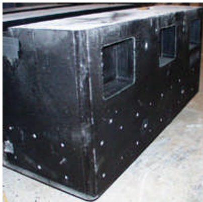
As-cast polymer composite base for high-production automated groove and trim machine (left), and finished machine being rigged for shipping.
